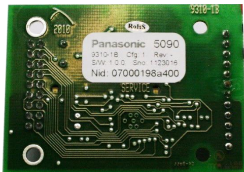
5090 backside The unique Neuron ID number is printed on the label.
