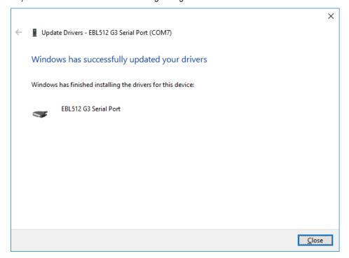
o) Before clicking Close, make a note of the COM-port number shown in the title row of this dialog (COM7 in this case). This COM-port number should be used in EBLWin / EBLFirmwareManager when logging on or downloading firmware to the control unit
