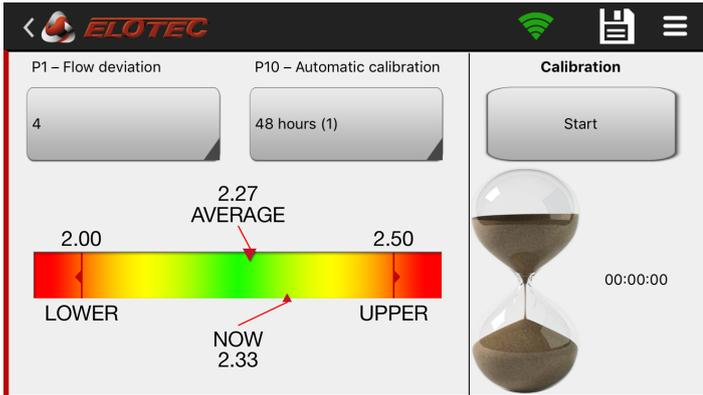
Log on to the Aspect with the Aspect tool - make the hand shake (green sleeves). Press the button below the Calibration header to start the process. The initial calibration will take about one minute, and the remaining calibration time is displayed to the right of the hourglass. After calibration, arrows should be in the green area.
