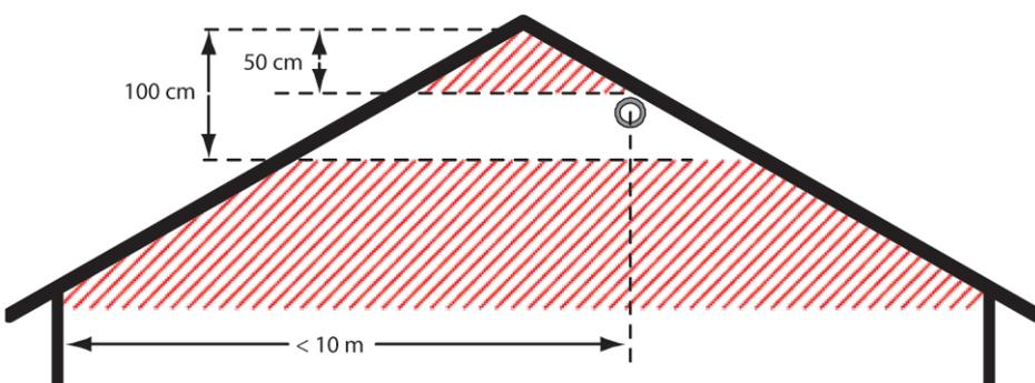
Installation of pipeline under a gable roof. Proper distance from the ridge is important.
