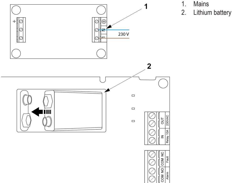
Connect the 230V mains on the right-hand side of the mains filter in the top of the device.
