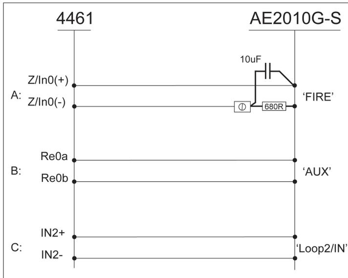
An alarm resistor is required for the stand-alone Aspect to fulfil EN54-13.
