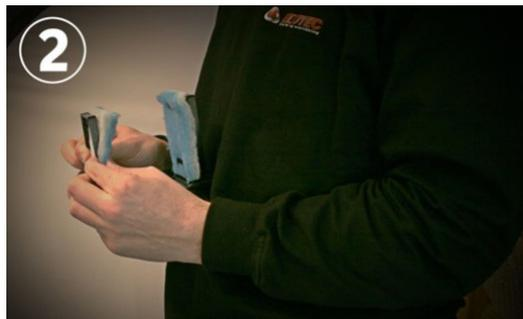
Finally, reinstall the cartridge, making sure that it is fitted tightly. Use your thumb to feel that the cartridge front is flush with the two raised areas of the filter housing.
