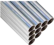
**According to VdS/EN54-20, pipe parts must comply with EN61386-1, at least class 1131. Use only approved original Elotec pipes that fulfil additional demands to rigidity (prevents drooping) and surface finish.**
