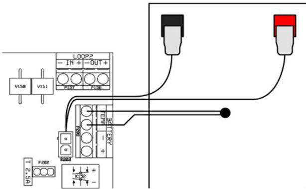
*Take proper care of the battery. Lead batteries can be damaged by deep discharge, so if a long-lasting power outage drains the battery completely, it may have to be replaced. If the battery is disconnected for some reason, self-discharge will permanently reduce its capacity if it is not recharged within 6-9 months. Standard batteries have an expected lifetime of no more than five years, and must be replaced every 3-5 years.*
