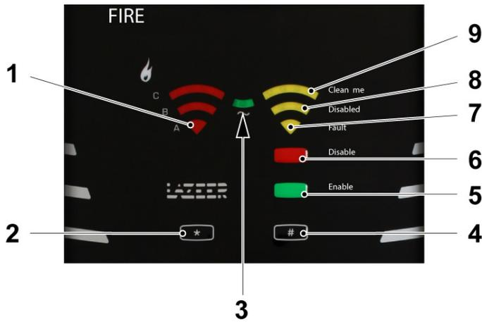
1. Red LED on – Smoke detected. Increasing amount is indicated by A/B/C.
