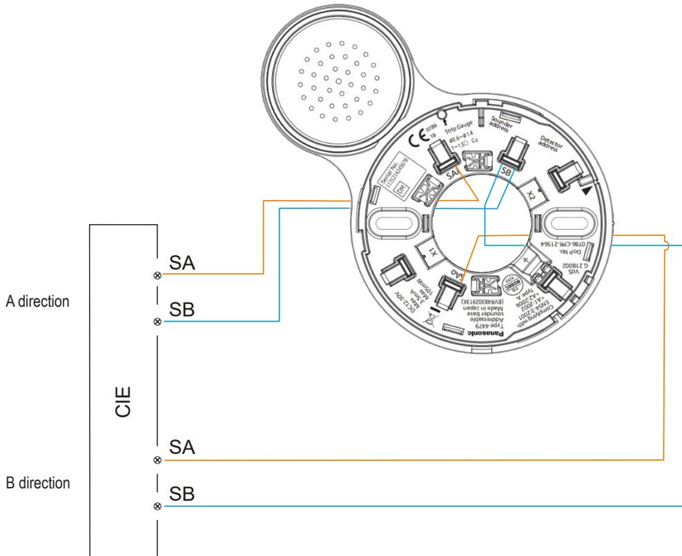
The base is prepared for mechanical locking of the detector when a detector with a locking screw is plugged into the base. Analog detector with isolator 4400I must be plugged in the addressable sounder base 4479.
