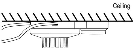
If the sounder base is mounted with the cabling entering from above (through the inner ceiling), there is a need for an ingress protection (type 4489).
