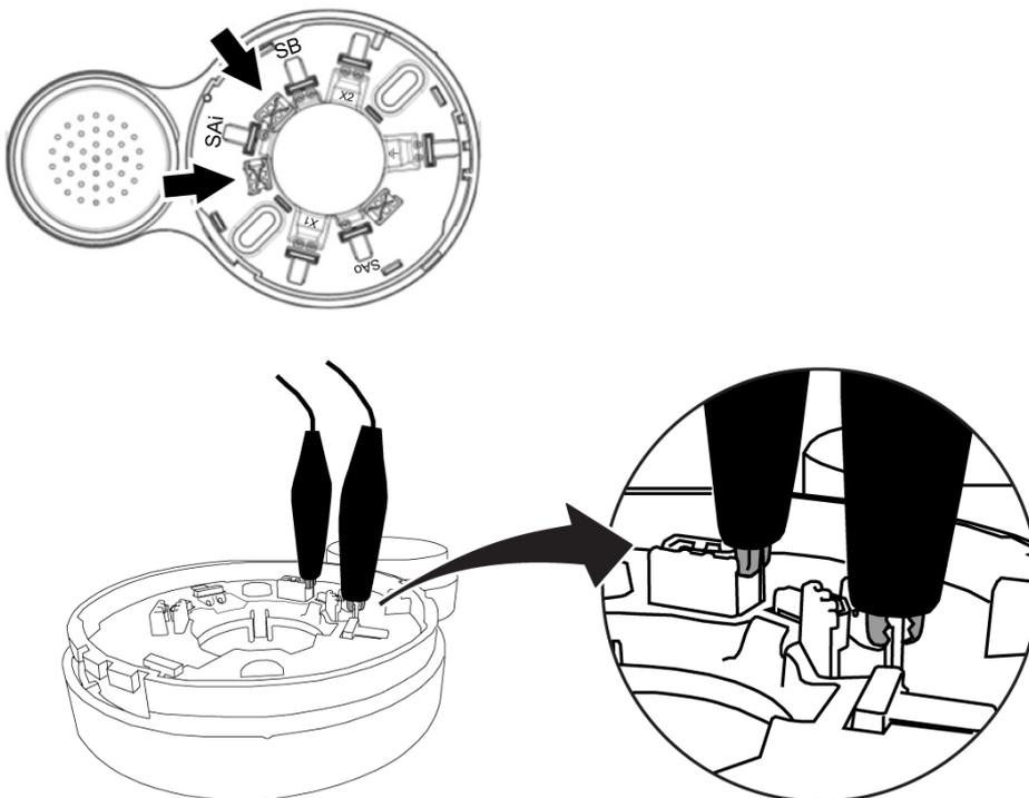
*The COM loop address and mode settings have to be done before the unit is connected to the COM loop.*
