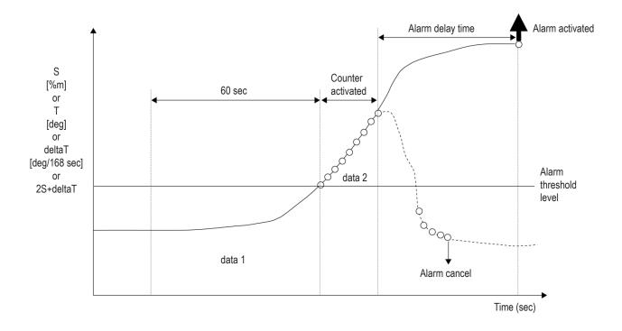
Maximum alarm delay time is 60 seconds.
