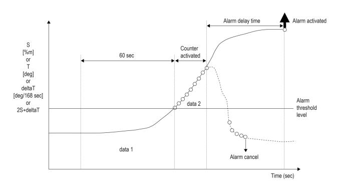
Maximum alarm delay time is 60 seconds.
