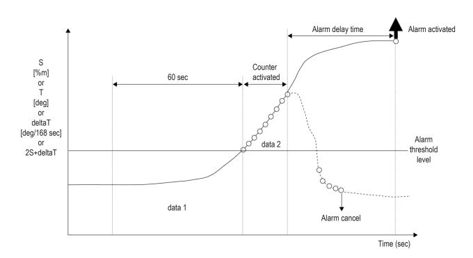
Maximum alarm delay time is 60 seconds.
