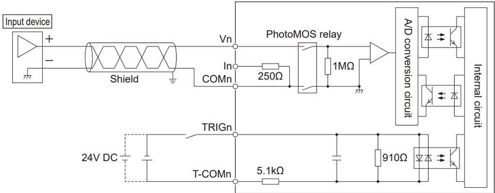
**■ Terminal layout (For voltage input)**
