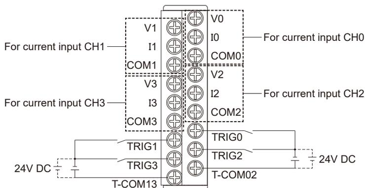
(Note 1) TRIG0 to TRIG3 of AFP7AD4H indicate input terminal numbers. Note that they do not correspond to the analog inputs "CH0 to CH3".
