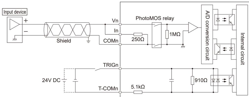
(Note 1) For the current input, connect the V and I terminals.
