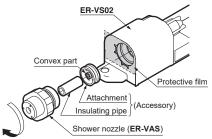
Note: Be sure to fit the insulating pipe and the attachment. When they are not fitted, the static removal capability remarkably deteriorates.
