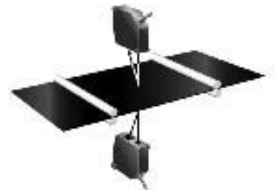
Measuring the thickness of rubber sheet
