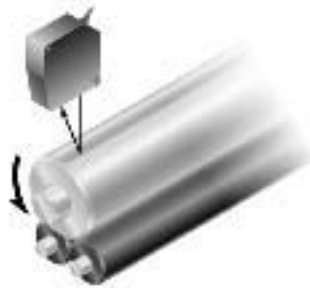
Detecting the seams of a metal drum
