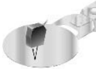
Measuring the eccentricity of a metal shaft
