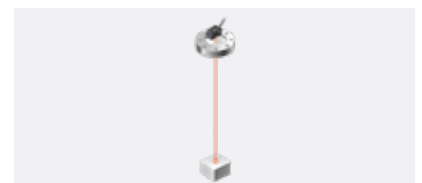
Detection of parts through viewing port
