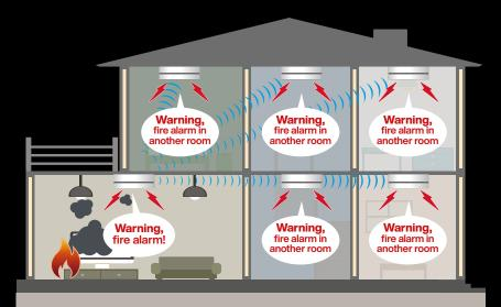
With Panasonic's product, when one smoke alarm goes off, then all the other alarms will also go off with different voice messages to warn all the residents about fire. Simply install a smoke alarm in each room and pair each device with the master smoke alarm in one of nine languages.
