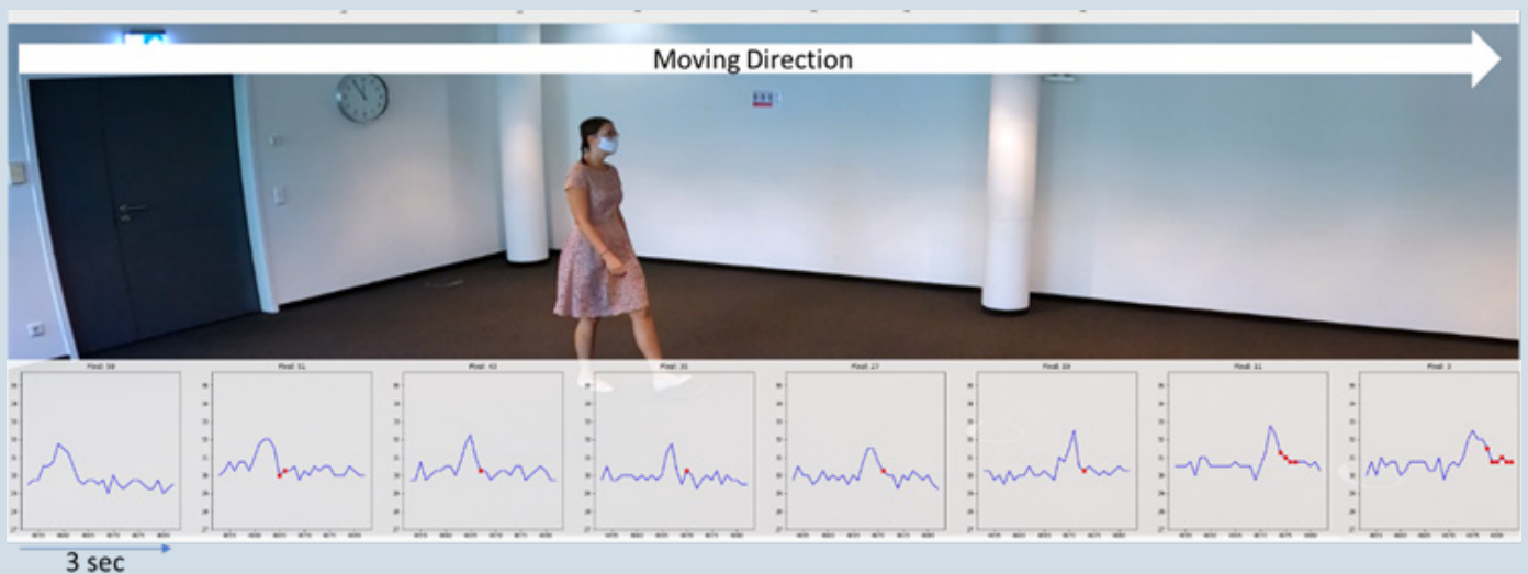
Figure 14: Walking person, Measurement data for one row of 8 Pixels. X-axis shows the time in 1/10 sec steps, the y-axis the raw temperature in degC. The red dots in the chart is showing a detected person.
