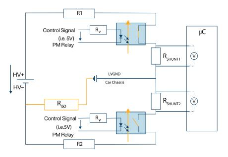
HV+ and HV- and thus, there is a certain current flow in the corresponding path. Due to that current through the Shunt resistor (RShunt1 and/or RShunt2) a respective voltage drop is detected by the control electronics and as a result a cutoff function for the traction battery is activated.
