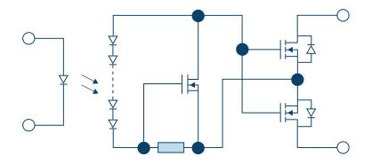
The MOSFET's capacitances and their time constants influence not only switching times, but also the output's isolation characteristics for higher frequency load signals. Essentially, they act as a reactance with a frequency-dependent value: The reactance is high for lower frequencies and decreases with rising frequencies. This can cause higher-frequency load signals to leak through the off-state output.
